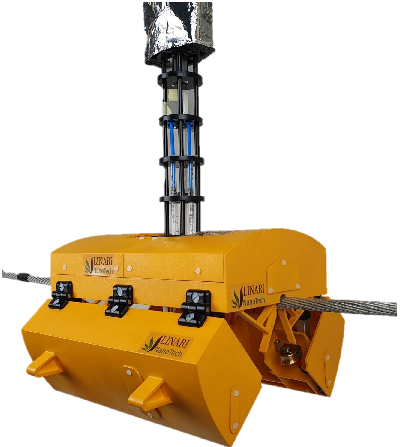
Figure 1: Nanofix during take-off / landing on electric line, lateral view
