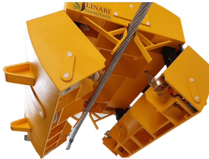
Figure 2: Nanofix during landing on electric line, bottom view
